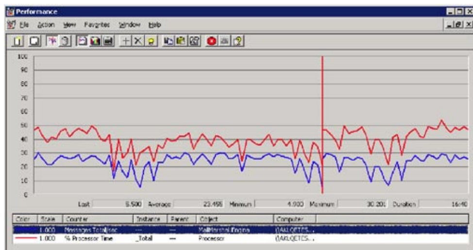
Figure 9 - MailMarshal 5.5 message throughput: 16 min window with a 10 sec sample
