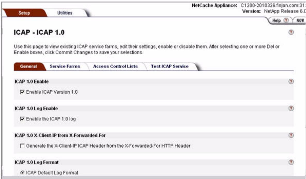
Figure 4-3: ICAP Setup - General
