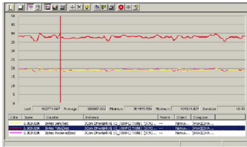
Figure 5 - Standalone server internet bandwidth utilization, 16min window with a 10sec sample
