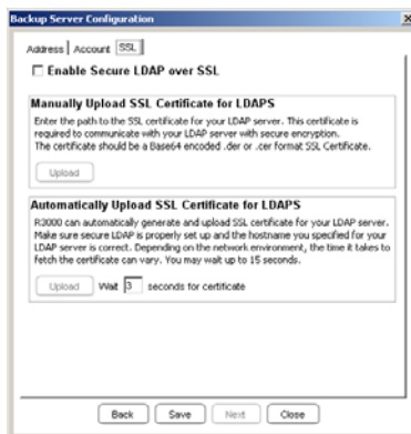
Fig. 3-16 Backup Server Configuration, SSL Settings
